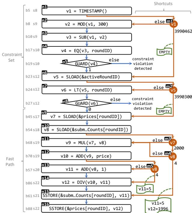
**Figure 8.** Accelerated program of  $Tx_e$  synthesized in FC1. All the variables whose names do not start with  $v$ , such as  $roundID$ ,  $\&activeRoundID$ , are constants. The corresponding line numbers in EVM trace and the source code are annotated in the left two columns.
